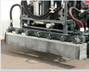
Insulated binder tank with various options, e. g. auxiliary electric heater, electro-pneumatic individual nozzle control, rear mounted working headlight etc.
