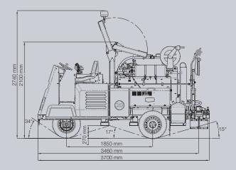
Self-propelled spraying machine **WEIRO® TM 800 SH** with a net capacity of 800 I to ensure the reliable layer bonding with polymer modified binders, i. e. according to TL BE-StB 15 (bitumen emulsion) and tack coat binders, equipped with ROPS (foldable), certified according to DIN EN ISO 3471:2010-01
