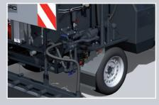
Self-propelled bitumen sprayer on extremely manoeuvrable 3-wheel chassis for the reliable and accurate application of all kinds of cold-liquid tack coating materials and bitumen emulsions, including polymer modified binders
