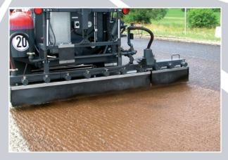
Leading to quality: accurate binder spraying by computer assisted automatic dosage system (option), even spray pattern through advanced spraybar design
