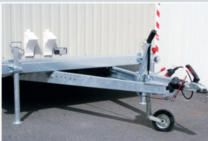
chassis made from galvanized lightweight profiles, galvanized prop stands
