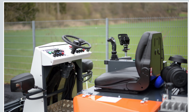
Ergonomically designed driver's place with joystick for electric drive control. Additional work light for best illumination of the working area.
